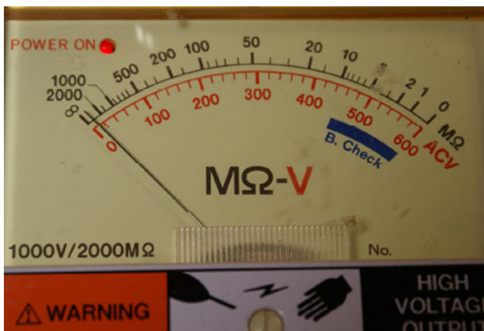
Our loop reading over 2000 MΩ, even under such extreme conditions.
